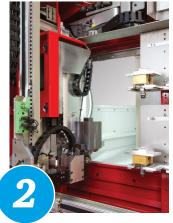
Simple Automation (option) For customers with small component sizes and small batch sizes the 30 position integral magazine will be very attractive, this unit fits under the tool magazine pallets and can change workpieces up to  $70 \times 70 \times 150$  mm high.
