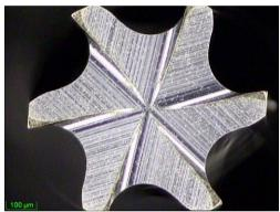
Examples of the endface of a 0.8 mm diameter endmill in a new condition (top) and when the tool had been used (bottom). Evaluation of the tool wear helps the operator to decide on the estimated tool-life remaining.
