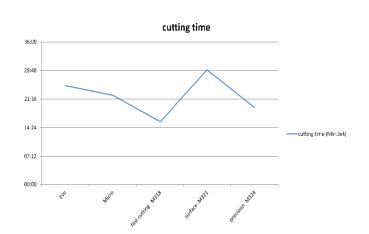
It can be seen that when using the M-Code for fastest production speed the cycle time is approximately 15 minutes while to achieve the best surface finish the time is 28 minutes – all by using one simple command.
