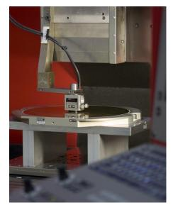
KERN, being a German machine tool manufacturer, uses VDI/DGQ3441 as a standard for the measurement of accuracy on their range of machining centres. Positional accuracy (Ps) is  $\pm 0.0005$  mm. Attached are axis measurement certificates for all three axes, X, Y and Z.
