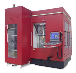
Automatic workpiece changing systems are available and can be retro-fitted at a later date. There are 3 types of palletisation system:
