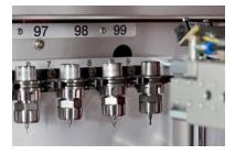
Whether HSK25 or HSK40 the maximum tool length (including the tool holder) is 150 mm. While a maximum diameter of 70 mm is possible with adjacent tool positions vacant in
