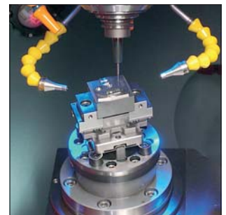
Ultra precision machining in hardened steel 47 HRC
