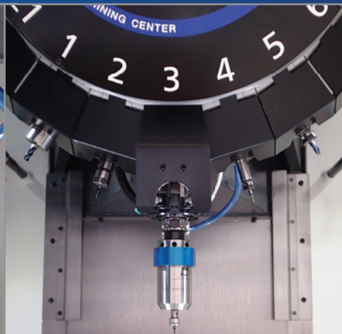
625XDT milling at 50,000 rpm, 0.80 hp
