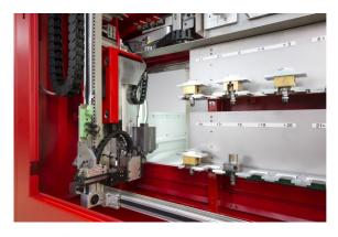
Automatic workpiece changing systems are available and can be retro-fitted at a later date. There are 3 types of palletisation system:
