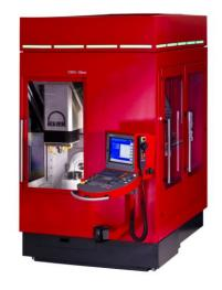
The KERN MICRO is an ultra precision machining centre with the highest level of accuracy in 5 axis configuration. The working envelope is 350 x 220 x 250 mm.
