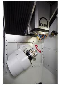
The machine working area is easily accessible through two sliding doors —one at the front of the machine and one to the left side, which are interlocked for safety when the machine is working in automatic operation. The Heidenhain iTNC control unit is also positioned on the front of the machine on a swivelling pedestal that reaches to the optimum position by the doors when setting-up.
