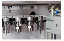
Whether HSK25 or HSK40 the maximum tool length (including the tool holder) is 150 mm. While a maximum diameter of 70 mm is possible with adjacent tool positions vacant in
