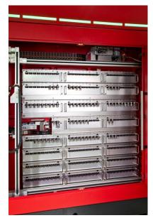
The tool cabinet is situated on the right side of the machine and the doors can be opened while the machine is working but a tool change is prevented by the machine operation safety system.
